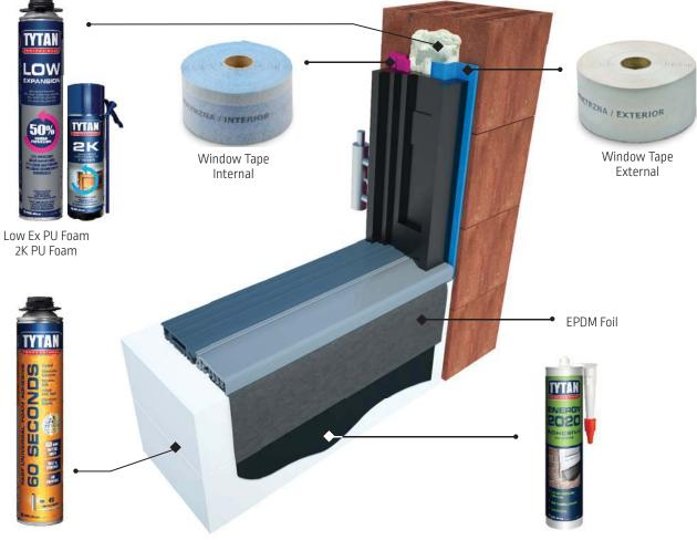
60 Seconds Fast Foam Adhesive Adhesive for EPDM Energy 2020
