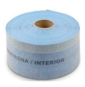
Window Tape Interior provides an additional insulating layer between the wall and frame of windows or doors, thus protecting the joints from absorbing the moisture from the room. The tape consists of a high quality vapour barrier membrane, which guarantees the optimum value of Sd  $\geq$  50 m, coated on both sides with non-woven polypropylene.
