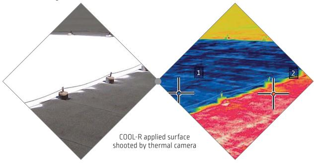
COOL-R reduces the roof temperature by 70%, and inside the building - up to 10°C
