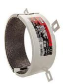
B1 Fire Collar is designed to maintain the fire resistance of fire rated walls and floors where these are breached by continuous plastic pipes, and may be used in gypsum, masonry and concrete walls and floors. The steel shell contains a graphite based reactive material which reacts when exposed to heat closing the openings left by the softening plastic pipe in fire.
