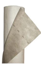
Three-layer vapor-permeable roof membrane. Made of two layers of polypropylene nonwoven and special functional polyethylene film which ensures high vapor permeability and water tightness of the underlay. Owing to its high vapor permeability, it can be applied directly on insulation and consequently a venting slot is not required between the membrane and the thermal insulation.
