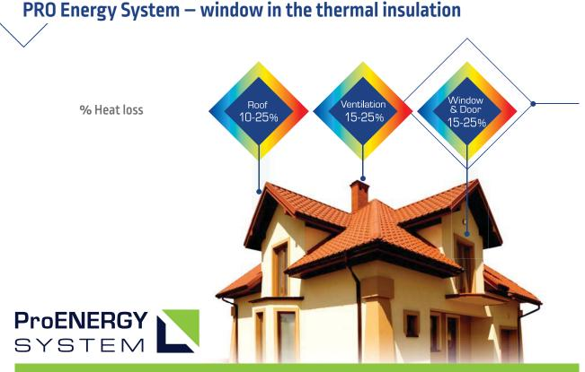
To reduce heat loss from the building you should not only ensure the selection of energy-efficient windows (with best U coefficient), but also correct installation and the use of high quality materials to insulate joint around the window. By using Tytan Window System we reduce the occurrence of fungi, mold and thermal bridges. The main three benefits of Tytan Window System are:
