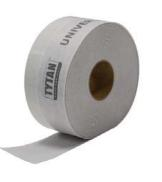
Universal tape for window & door installation, recommended for protection and insulation of connections between the wall and the frame of windows or doors, both inside and outside the building. The tape consists of a high-quality smart membrane with a variable Sd rate, which eliminates the need for two dedicated tapes.
