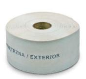
Window Tape Exterior provides an additional insulating layer between the wall and frame of windows or doors, preventing the joints from absorbing the rain and wind and improving the overall insulation parameters. The tape consists of a high quality vapour permeable membrane, which guarantees the optimum value of Sd  $\leq$  0,05 m, coated on both sides with nonwoven polypropylene.
